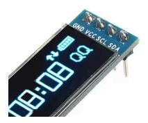
No Soldering is needed for the display, use the 4pin dupont cable:
