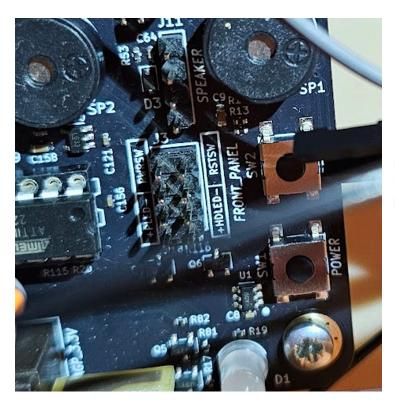
Power switch connect to PWRSW Reset Switch connects to RSTSW Polarity does not matter for these.
