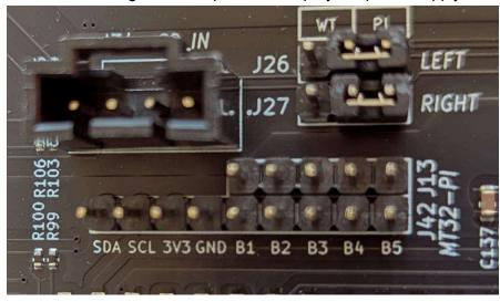
SYNTH switch goes to B1 and ROM switch goes to B2, i suggest keeping the black wire upwards on the J13 line of pins as that is the ground pins.
