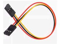
One end of the wire with the dupont connector goes to the llama board pin header below the ATX connector
