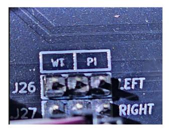
The Switch works "reversed", so when mounting it in the case when the toggle is in the down position, pointing at PI printed on the case, the wires in the top row will be activated, if function is reversed, just rotate half a turn.
