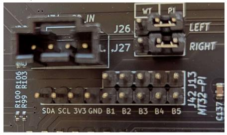
Connect it to the first four pins, be careful to connect the dupont connector in the right orientation. SDA=Yellow, SCL=Orange, 3v3=red, GND=Brown
