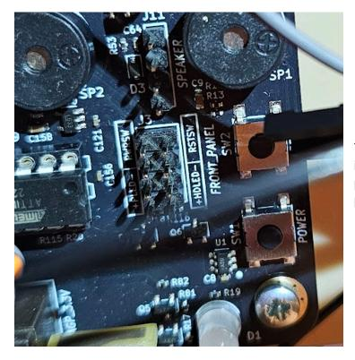
The dupont connector then goes into the +PLED- and the +HDLED-pins on the lama, do mind the polarity!
