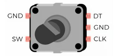
Do note that this image is seen from the front with the rotary shaft towards you. For this we use one 3wire cable with dupont connector and two 1wire dupont.
